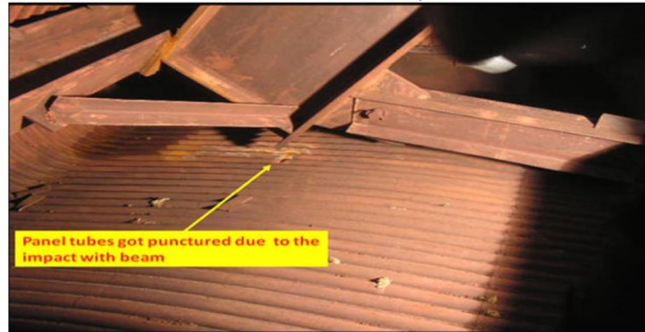
Location of failed tubes
