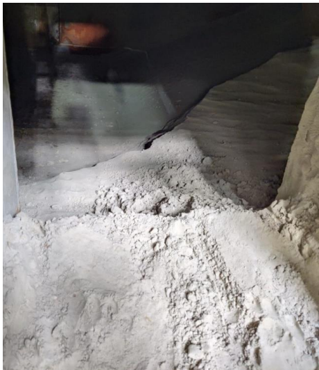
Ash Accumulation in the Windbox
