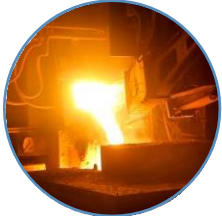
Flame instability due to high coal quality variations in domestic coal (High Ash, Low VM in Indian Coal).
